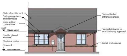
2 Front Elevation_Brick Scale: 1 : 100
