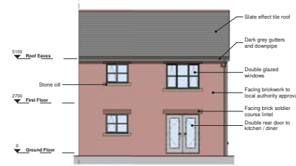
5 Rear Elevation_Brick Scale: 1 : 100
