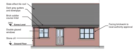
4 Rear Elevation_Brick Scale: 1 : 100
